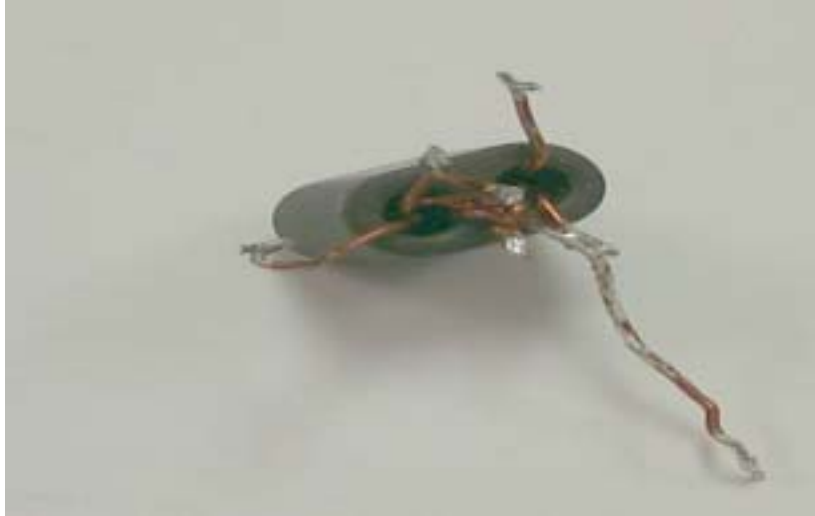
FIGURE 20: T1, 25:1, MULTI-FILAR AUTOTRANSFORMER
